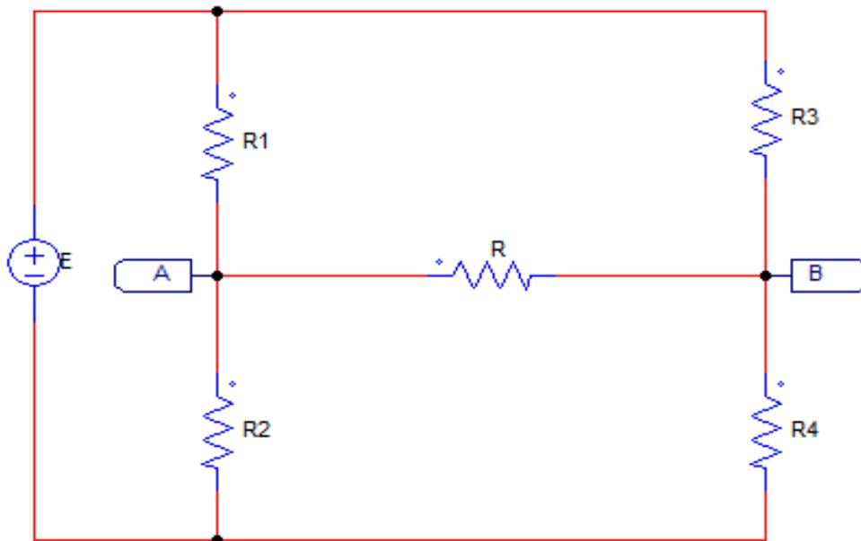
On donne :  $E = 240 \text{ V}$  –  $R_1 = 40 \text{ } \Omega$  –  $R_2 = 160 \text{ } \Omega$  –  $R_3 = 60 \text{ } \Omega$  –  $R_4 = 100 \text{ } \Omega$  –  $R = 10,5 \text{ } \Omega$
