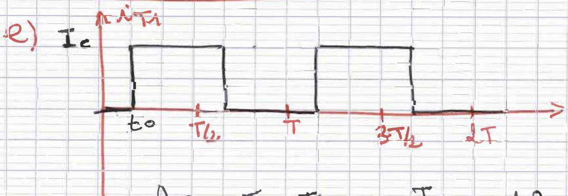
$$\langle I_{T1} \rangle = \frac{I_c T}{T} = \frac{I_c \times T/2}{T} = \frac{I_c}{2} = \frac{12}{2} = 6 \text{ A}$$
